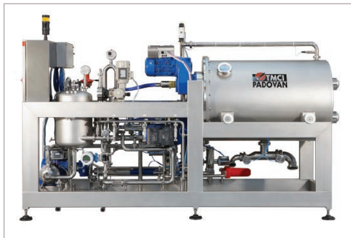
Padovan's Dynamos uses stacked, rotating ceramic discs that filter wine from the outside of the membrane to the inside and into a hollow shaft that runs down its center.
