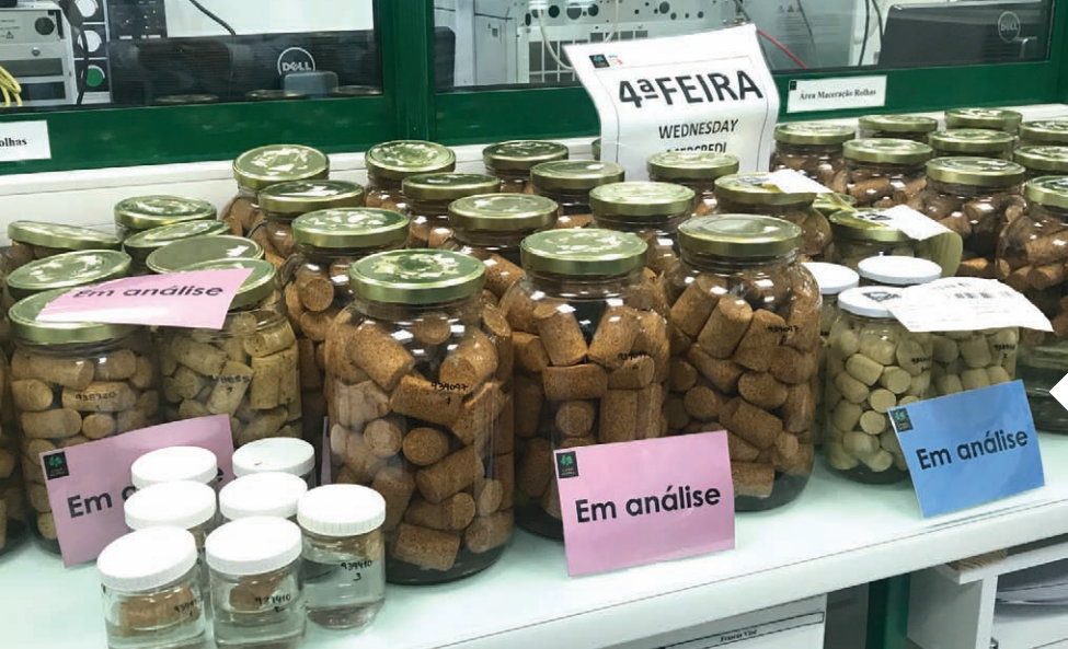
Cork samples soak overnight during TCA batch testing of various lots at Cork Supply.
